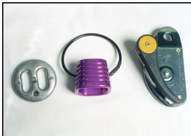
Figure 3-20. Slot, tuber, mechanical camming device.
