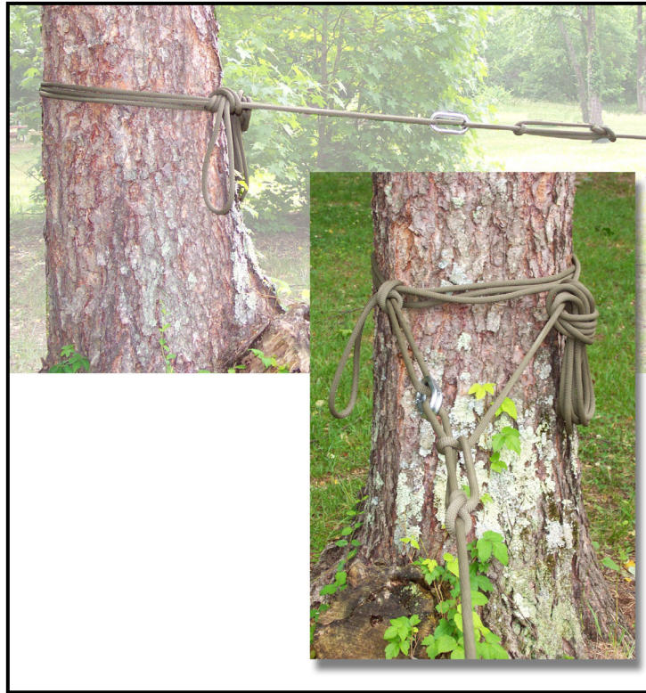
Figure 7-12. Round turn around anchor and two half hitches on a bight.
