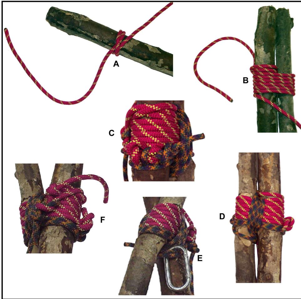
Figure 7-20. A-frame horizontal and vertical wraps.
