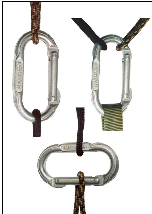
Figure 3-12. Major and minor axes and three-way loading.
