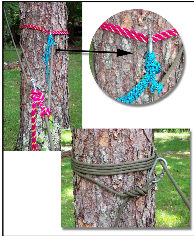
Figure 7-14. Z-pulley tightening system.
