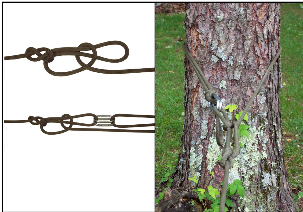
Figure 7-10. Transport tightening system.
