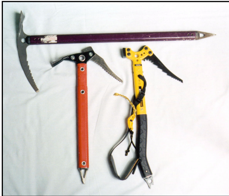
Figure 3-24. Ice ax and ice hammers.
