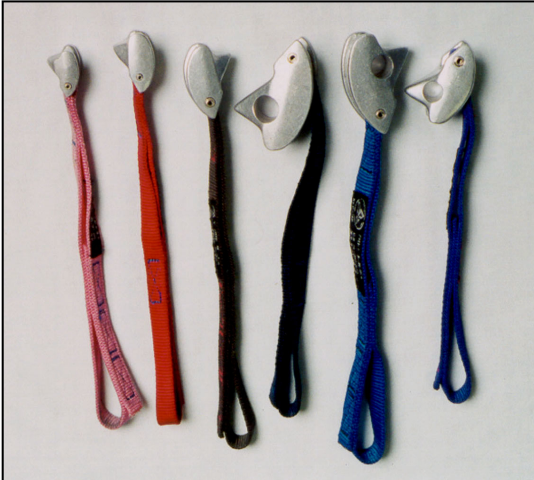
Figure 3-16. Three-point camming device.
