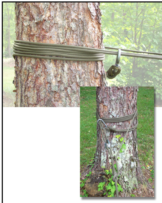
Figure 7-13. Tensionless anchor knot.
